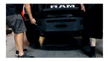
and attach with the provided 10mm T-Bolts. Insert the T-bolts through the mesh vent opening in the side of the bumper and through the bumper inside bracket and outside bracket. Do not fully tighten the T-bolts yet.
