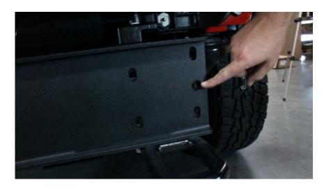
using the provided 10mm bolts and hardware. Install the bolts into the outer most holes in the winch carrier and fully tighten.
