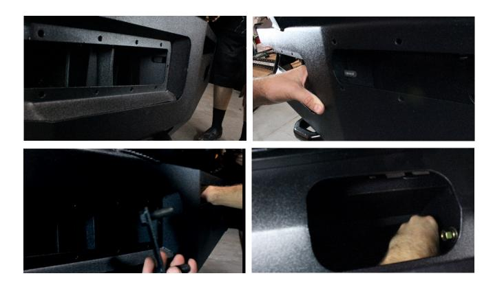
10. With the bumper loose fit on the truck, align the bumper side to side and front to back. Once aligned fully tighten all the hardware on all 4 t-bolts.
