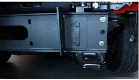
9. With assistance mount the Alumilite bumper onto the outside brackets
