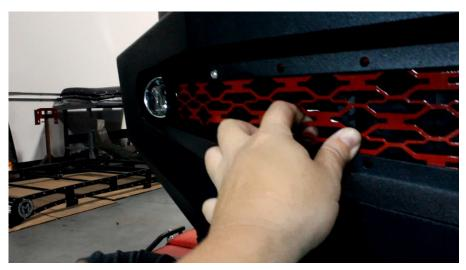
The center mesh panel is designed with tabs that will fit a Single Row 20 Inch LED Light Bar with Stud Mounts and Dimensions of L 21 5/8" x H 1 5/8" x W 3", behind the mesh, if desired.
