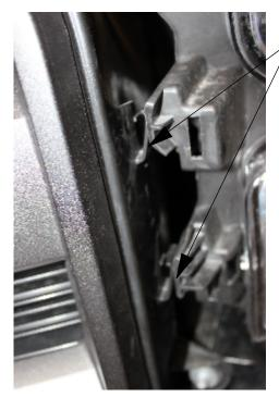
Step4 Grille retaining tabs two per side
